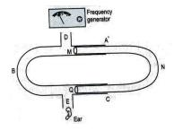
The sound generated by the frequency generator travels through DEB and DNE and super imposes at E. If the path difference between the above two paths is 0,  $\lambda$ ,  $2\lambda$ ,....  $n\lambda$  then constructive interference takes place at E and we get a sound of maximum intensity at E. If the path difference is  $\lambda/2$ ,  $3\lambda/2$ ,.....  $(2n+1)\lambda/2$  then destructive interference takes place at E and we get sound of minimum(zero) intensity at E.
